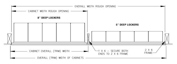
Side View of Cell Phone Lockers in Wall
