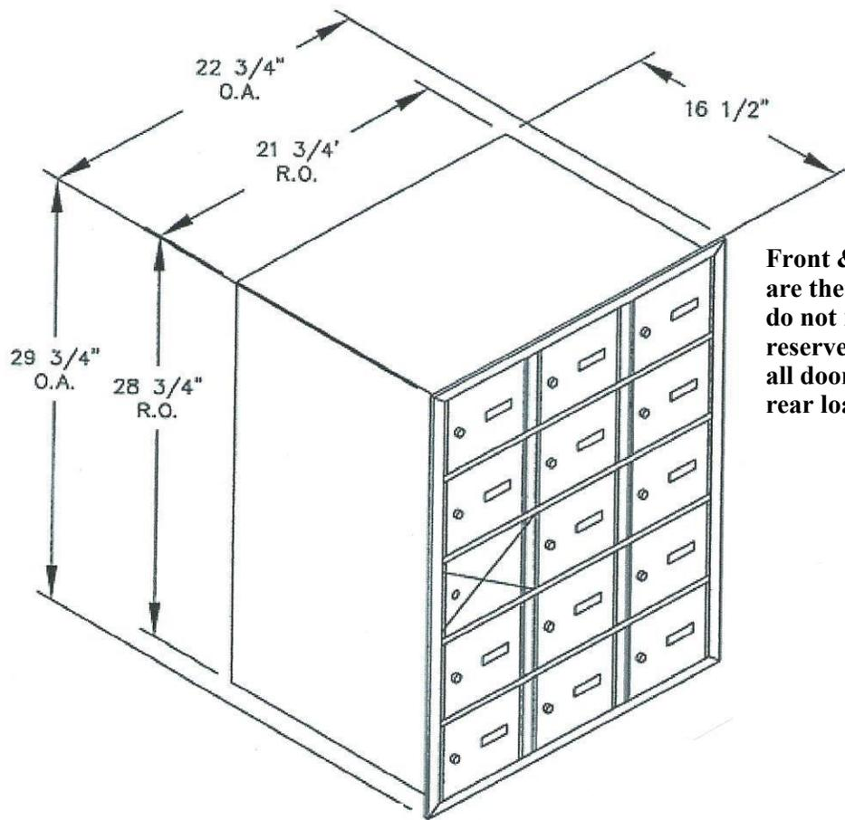
**Front & rear loading dimensions are the same. Rear loading modules do not require a master door to be reserved for master entry. Therefore, all door compartments are usable for rear loading modules.**
