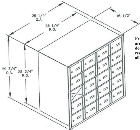
Front & rear loading dimensions are the same. Rear loading units do not require a master door to be reserved for master access. Therefore, all compartments are usable.
