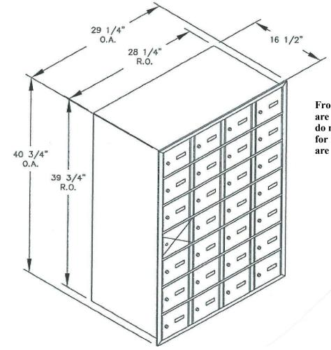
Front and rear loading dimensions are the same. Rear loading units do not require a door to be reserved for master access, therefore all openings are available for storage.
