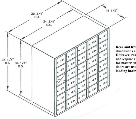
Rear and front loading unit dimensions are the same. However, rear loading units do not require a door to be reserved for master entry. Therefore, all doors are usuable for rear loading horizontal mailboxes.
