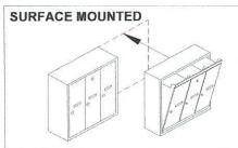
Units mount directly to a surface and are attached with mounting hardware through the back.
